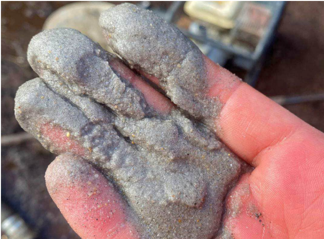
Fine sands (LTA) passing through the filter pack during development of BH-PB01
