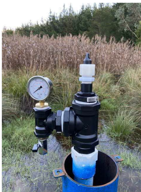
BRBH01 artesian well fitting with logger, gauge and outlet
