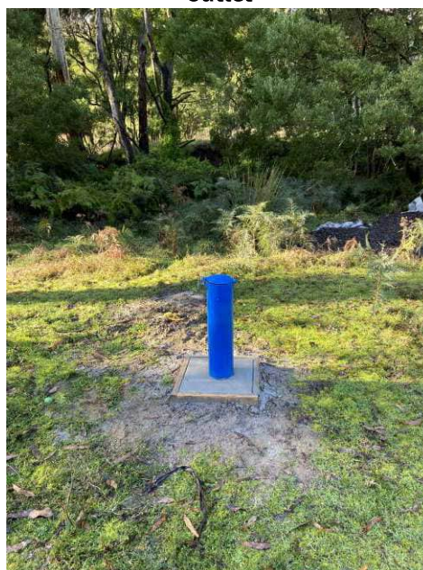
BRBH01 artesian well fitting with logger, gauge and outlet
